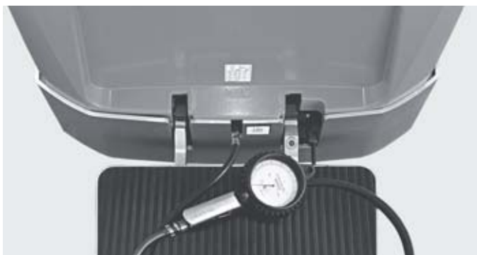
Protects the back: the air-cushioned stand-on platform can be adjusted to individual driver's weight
